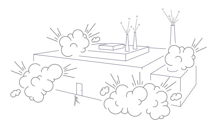
**Figure 3:**The dust cloud erupts and sends a fireball through the entire facility
